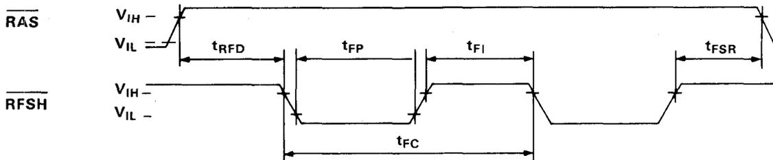
RFSH (PIN 1) COUNTER TEST WRITE CYCLE
